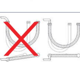
No torsion stress if using a double rigid pipe elbow.
