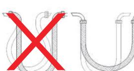
Correct installation only with rigid pipe elbow.
