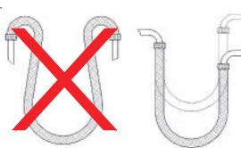
Correct installation only with rigid pipe elbow.
