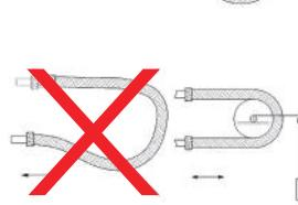
Use a movable coil to keep good position and in order to avoid variable movement and torsion.
