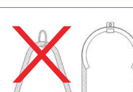
Using a saddle or a coil, buckling and consequently falling below the bend radius are avoided.
