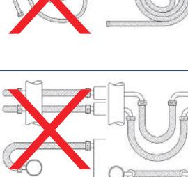
No torsion and favourable bending load thanks to the installation of rigid pipe elbows.
