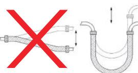
install rigid pipe elbows to avoid variable movements and too big bending load.
