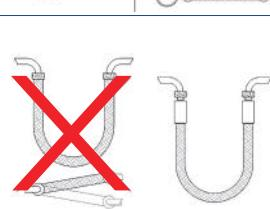
If torsion can not be avoided, use movable couplings which absorb torsion. Thus the hose is only exposed to bending load.
